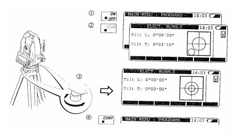
The instrument can be leveled up using the footscrews, without having to turn it through  $90^{\circ}$  /  $180^{\circ}$
